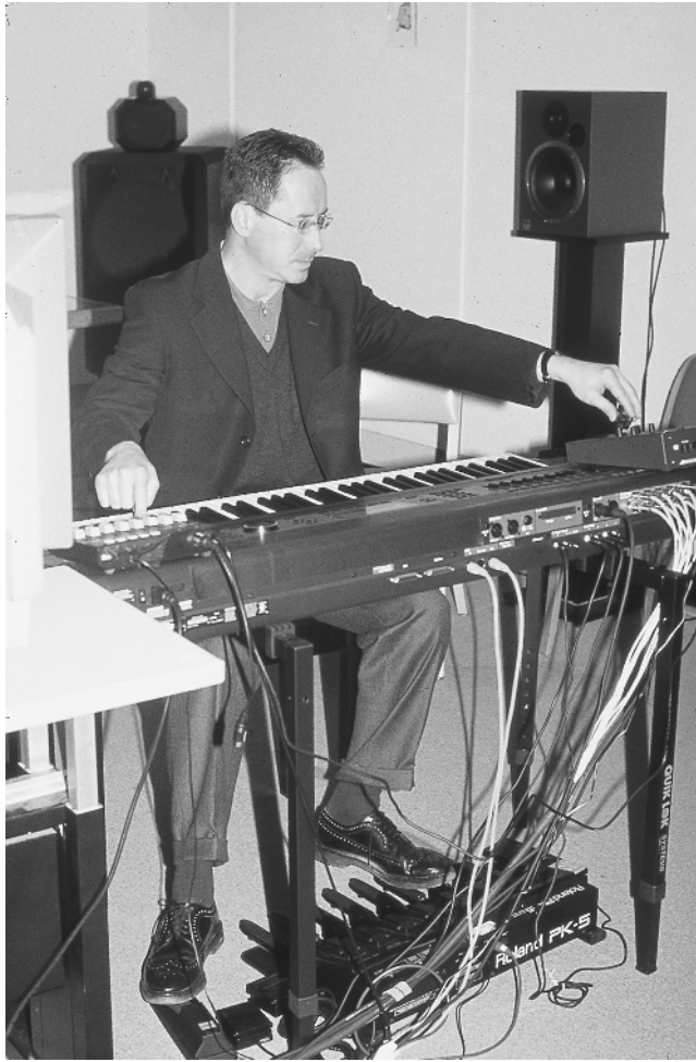
Figure 5.3 The author playing the Creatovox synthesizer in CREATE's Studio Varèse, January 2000. The physical hardware consists of a MIDI keyboard controller, MIDI joystick, and footpedals. A Power Macintosh computer receives the MIDI data. The Creatovox software interprets the MIDI data and synthesizes the sound, with octo-phonic output through a Digidesign Pro Tools 24 converter.
